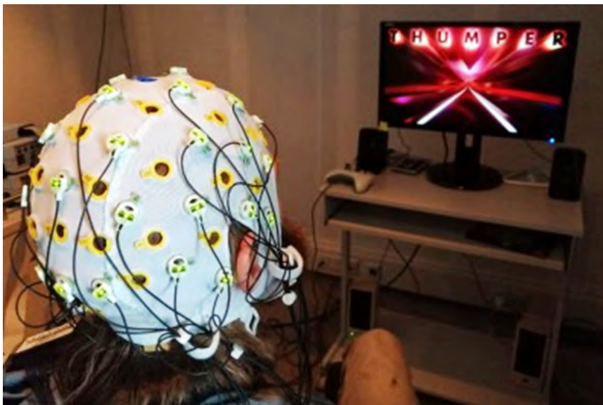
Fig. 13. A participant plays the commercially available video game Thumper. The detection of brain waves is undertaken with the EEG in order to assess the neural correlates of flow experience.
